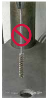
Incorrect Mounting in Chuck
