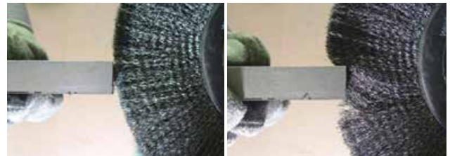
Correct Wire Tips Doing the Work
