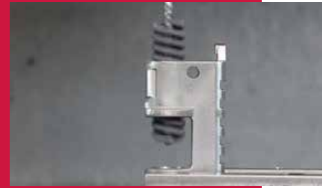
Deburring cross holes in a firearms component.
