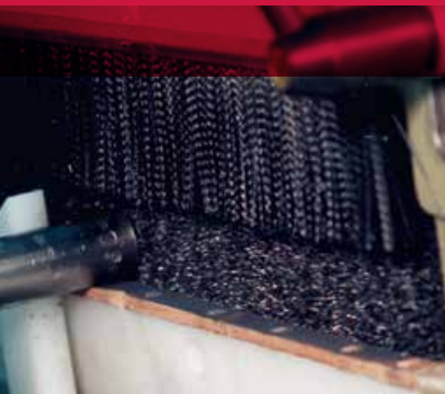
Straight strip brush used as a guard to prevent chips from flying.
