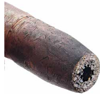
Nozzle fully clogged (not using E-WELD Nozzle)
