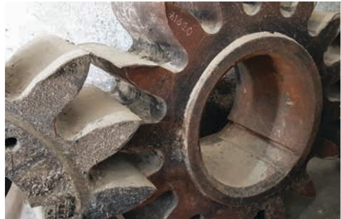
Sugar Mill Sprockets can be repaired with Stooddy 1105 and Super Build Up.
