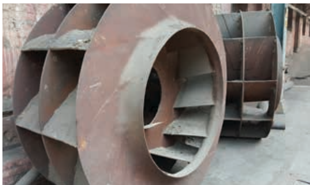
Sugar mill incinerator exhaust fan critical wear zones can be hardfaced with 87 TG oxyfuel torch powder.
