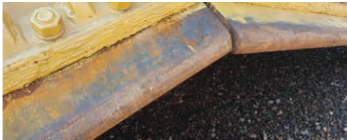
Stoodly 965 with addition of dropped tungsten carbides.
