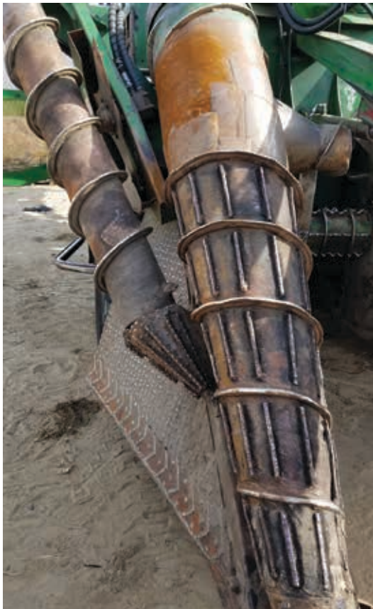
Stoodly 964AP-G applied to sugar cane harvester shoe.
