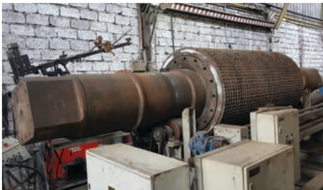
Stoody 600 and Stoody 101HC applied to sugar mill press rolls in Peru improved service life between hardfacing reapplications by 40%.
