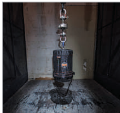
INVERTED STATIC TESTING Containers designed to carry contents that cannot be tethered should have a top or closure that is tested upside down to a 2:1 safety factor.
