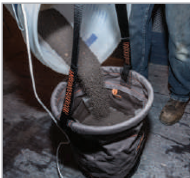
STATIC TESTING Portable and stationary containers should be statically pulled or loaded with a 5:1 safety factor.
