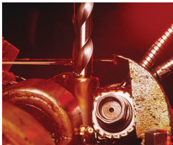
Flute milling of large diameter twist drills
