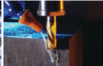
Profiling Involves Cutting Along The Edge Of The Material
