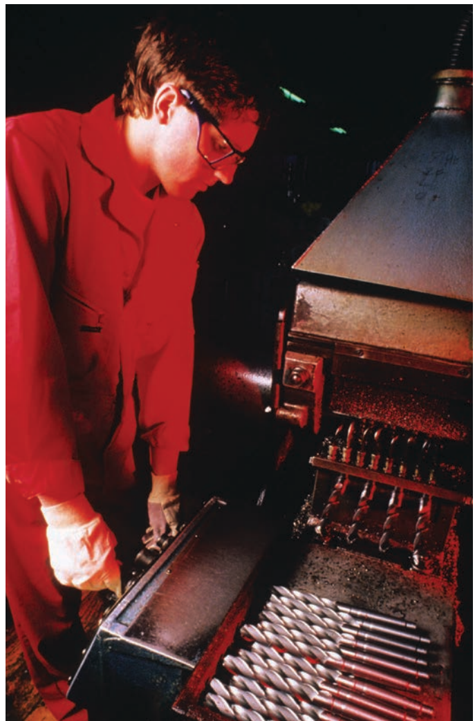
Flute milling of taper shank drills
