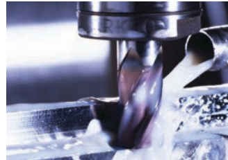
Profiling Involves Cutting Along The Edge Of The Material
