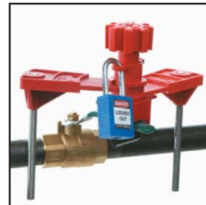
Use two blocking arms to lock out 3-, 4- or 5-way valves, or to lock in the ON, OFF, or throttled position
